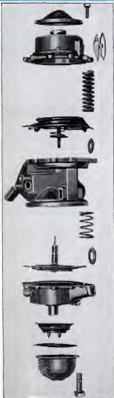
Below left, is exploded diagram of combination fuel pump-vacuum booster. Above left, assembled unit is shown with parts named. Drawing, above right, is cross section with all parts lettered for reference
